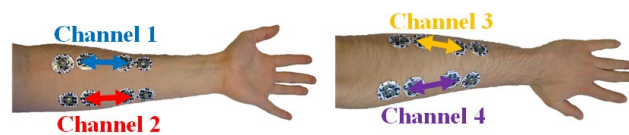
Fig. 12. Positioning of the 16 Ag/AgCl gel electrodes for performing measurements with four measurement modules. The distance between related voltage electrodes is about 4 cm.
